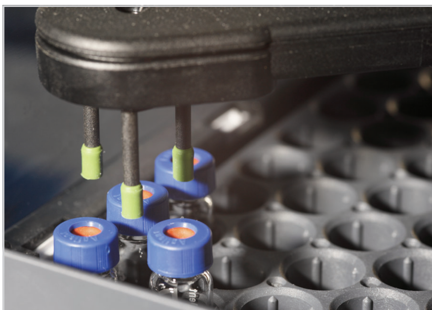
Automatic sampling systems allow for efficient storage and handling of a diverse range of clinical samples.
